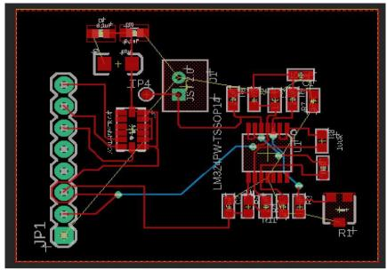
Figure 3 - GSR and 3-axis accelerometer board layout
