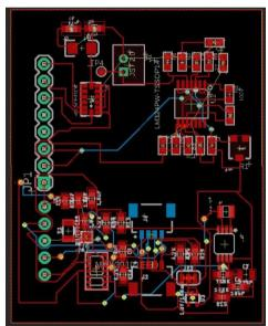
Figure. 4 GSR, PPG, 3-axis accelerometer board layout
